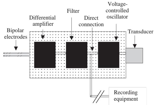
Fig. 1. Schematic diagram of the EMG tag components illustrating the bipolar electrodes (the insulation is removed 1 mm from the end), the differential amplifier, the filter, the voltage-controlled oscillator and the ceramic transducer. Also shown is the direct electrical connection at the output of the filter. A full circuit diagram can be obtained from M. Deffenbaugh.
