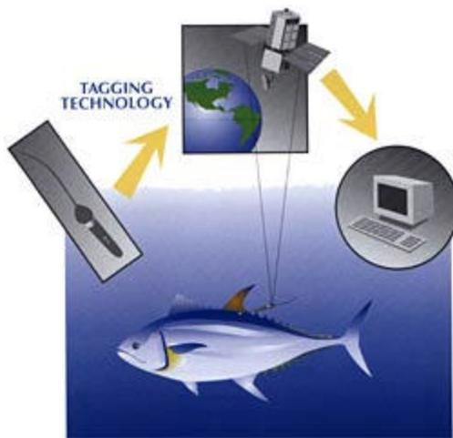
**Once a tuna is caught, a Pop-up Satellite Archival Tag (PSAT) is attached near the tuna's dorsal fin and the fish is released. The tag records the tuna's position every two minutes for up to a year. At a pre-programmed time, the tag is released, floats to the surface then uses cellular-phone technology to send the data up to a satellite. The information is then sent as an e-mail to a researcher's computer.**
